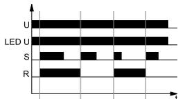
The input of the time relay is supplied with U voltage continuously. Closing of the control contact S immediately switches on the output relay R. Each next closing of the control contact S results in a change of the status of the output relay R to an opposite one (the feature of a bistable relay).
