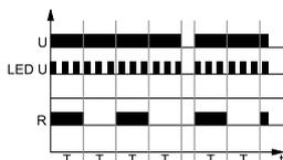
Applying the supply voltage U starts the cyclical operation from switching on the output relay R for the set interval T. After the interval T has lapsed, the output relay R switches off for the interval T. The cyclical operation lasts until the supply voltage U is interrupted.
