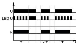
Applying the supply voltage U immediately switches the output relay R on for the set interval T. After the interval T has lapsed, the output relay R switches off.
