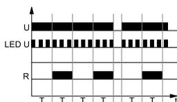
Applying the supply voltage U starts the cyclical operation from the interval T - switching the output relay R off followed by switching on the output relay R for the interval T. The cyclical operation lasts until the supply voltage U is interrupted.
