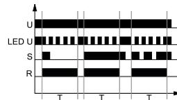
The input of the time relay is supplied with voltage U continuously. Closing of the control contact S immediately switches the output relay R on for the set interval T. After the interval T has lapsed, the output relay R is switched off. In the course of the interval T, any opening of the control contact S does not affect the function to be performed. The output relay R may be switched on again for the set interval, after the interval T has lapsed, by closing the control contact S again.
